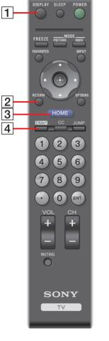
To operate this Internet Video Link receiver, use your Sony TV's remote control equipped with the **DMe<sup>x</sup>** button. If your TV's remote control does not have this button, your TV is not compatible with this receiver.
